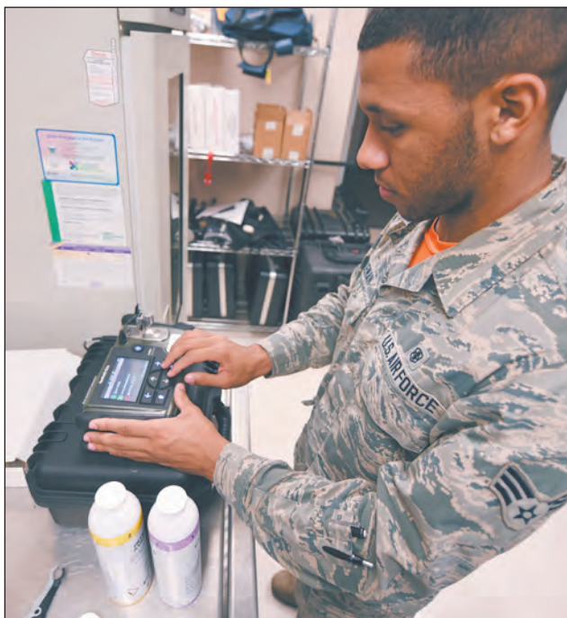
U.S. AIR FORCE PHOTO BY SENIOR AIRMAN HARRY BREXEL U.S. Air Force Senior Airman Emery Coleman, 19th Aerospace Medicine Squadron bioenvironmental engineering technician, uses a Hazardous Material Identification System to check a sample of soil for contaminations March 24 at Little Rock Air Force Base. Bioenvironmental engineering technicians respond to terrorist attacks, natural disasters and accidents to identify potential health hazards.
