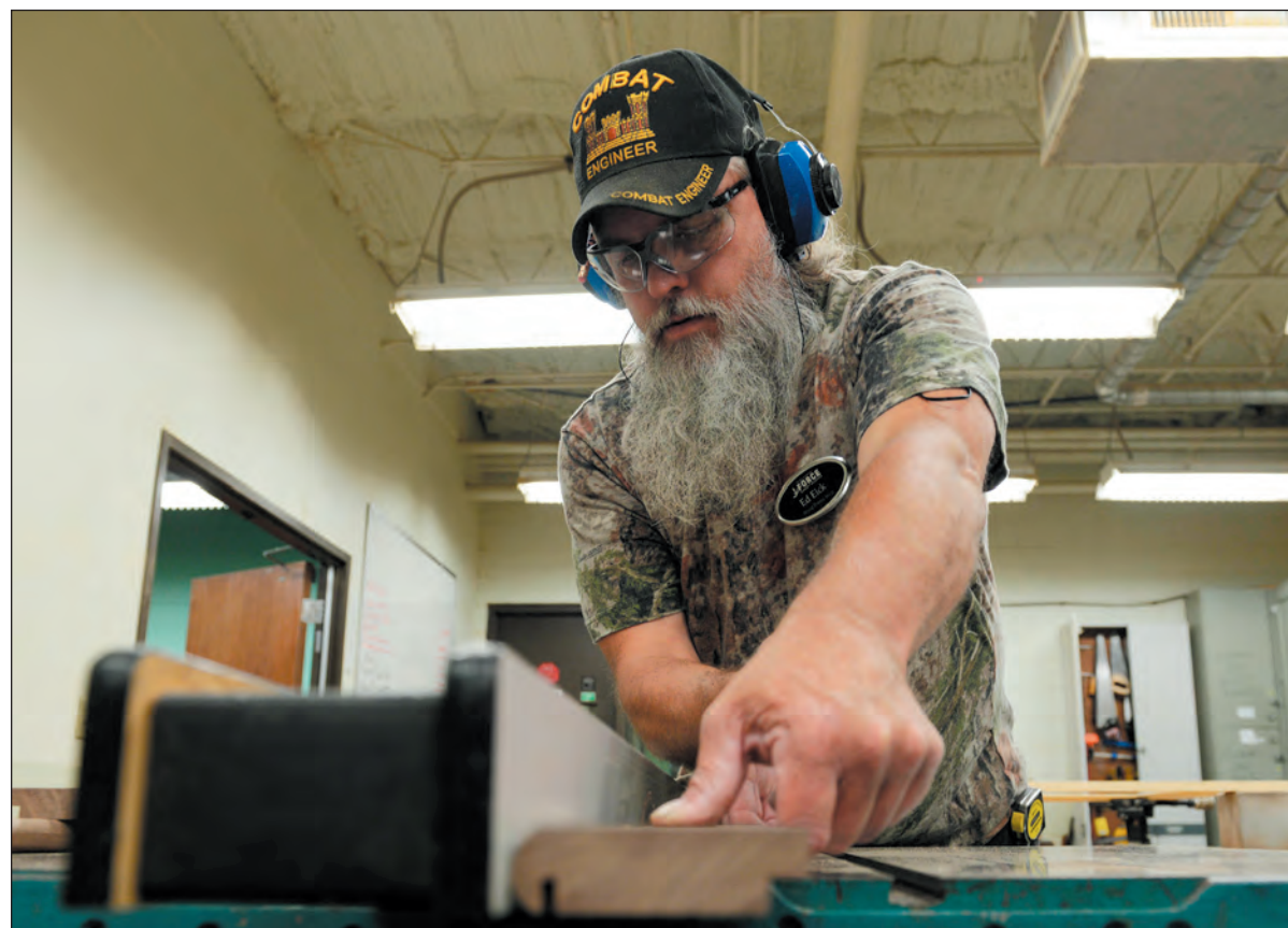
Ed Eick, 19th Force Support Squadron wood and frame shop worker, saws a slot in a piece of wood to allow glass to be placed inside, July 6 at Little Rock Air Force Base. Eick said that after 27 years in the military he puts a lot of heart and care into his work.
