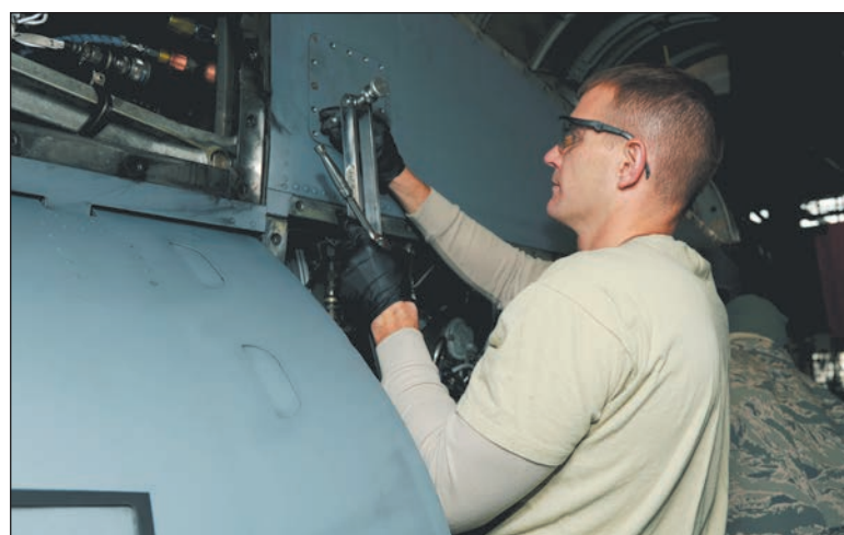
Tech. Sgt. Thomas Spuhler, a 19th Maintenance Squadron aerospace propulsion craftsman, removes a fuel nozzle access panel Nov. 13 at Little Rock Air Force Base. Spuhler removes the access panel to do a routine check on the fuel nozzle.
